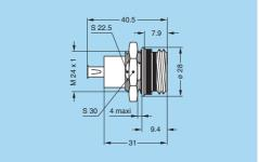
EG•.LM.U2A.XPL Fixed socket, nut fixing, key (W) or key (R)
