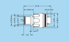
EG•.LM.U2A.XPP Fixed socket, female to female, nut fixing, key (W) or key (R)
