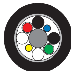
Riser grade HDTV cable
