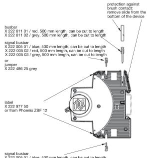
signal busbar X 222 005 01 / blue, 500 mm length, can be cut to length X 222 005 02 / red, 500 mm length, can be cut to length X 222 005 03 / grey, 500 mm length, can be cut to length
