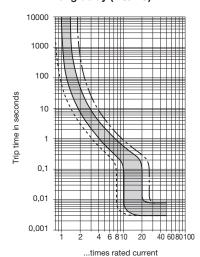
Magnetic tripping currents are increased by 30 % on DC supplies.
